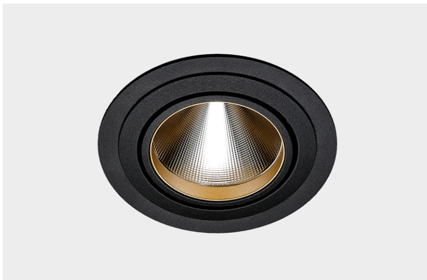
A new range of recessed directional LED fixtures. Cooled with passive heatsink. The LED unit can be rotated horizontally with 355° and tilted vertically. Various shapes in single, double or triple configurations form a wide range of options in round, rectangular or dipped frames. Various accessories and colour combinations, including metallic gold, enable you to customize the experience and to create an atmosphere that underlines the exclusivity of the installation.
