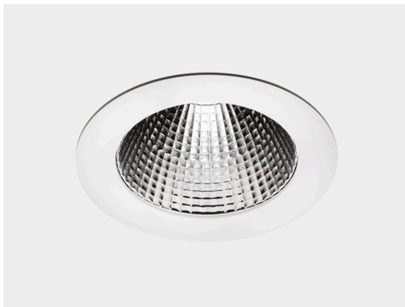
The Fry range is a basic and cost-efficient range of fixed LED downlights. The Fry 111 series covers the output range from 1200lm to 5000lm, all available in spot, medium and flood beam, in 3 colour temperatures, with a fixed output driver or a DALI driver and in 3 different finishes: white, grey or black. A smaller sized variant, Fry 70, covers the 1200lm to 3000lm output range.
